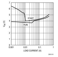
(6a) LT3502A Typical Minimum Input Voltage,  $V_{OUT} = 3.3V$
