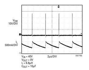
Figure 8a. The LT3502A Reduces its Frequency to Below 250kHz to Protect Against Shorted Output with 40V Input
