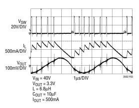
Figure 3. Pulse Skip with Large Load Current Will be Limited by the DA Valley Current Limit. Notice the Flat Inductor Valley Current and Reduced Switching Frequency
