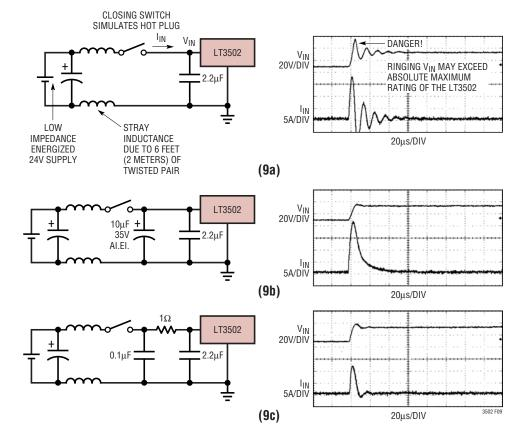
Figure 9. A Well Chosen Input Network Prevents Input Voltage Overshoot and Ensures Reliable Operation When the LT3502 is Connected to a Live Supply
