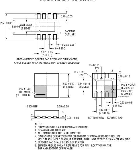
DC Package 8-Lead Plastic DFN (2mm × 2mm) (Reference LTC DWG # 05-08-1719 Rev Ø)
